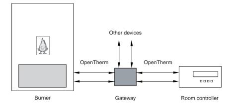
Figure 1-2: Block Diagram 2
