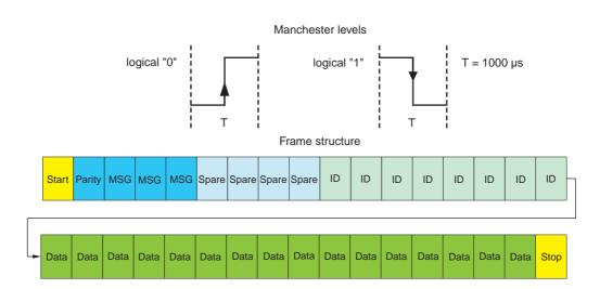
Figure 1-4: OpenTherm Protocol Frame Timing
