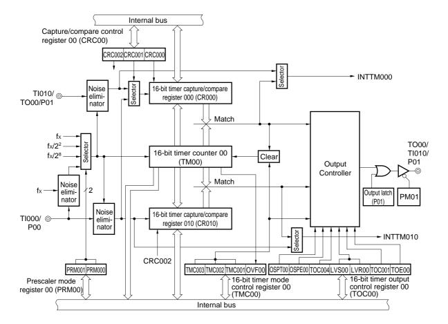
Figure 2-2: 16-bit Timer Block Diagram
